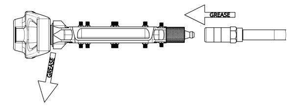
5. Screw the end cap back onto the pedal with 3Nm.
