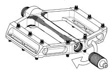
3. Take a grease gun and connect it to the grease nipple. Pump grease into the pedal until grease comes out of the other end of the pedal.
