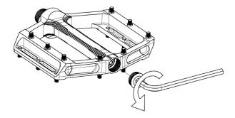
2. Screw the grease adapter onto the pedal by hand.
