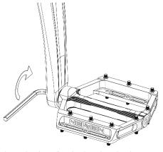
5. Now install the left pedal on the left (brake-) side. The letters for the respective side are shown on the inside of the pedal axle.
